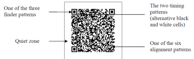
Fig. 11. The finder patterns, timing patterns, alignment patterns and the quiet zone of a QR code.
